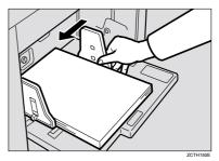
**3** When you finish prints, shift the feed roller pressure lever to the Standard paper position.
